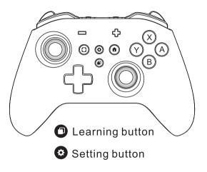
Controller automatically shuts down in case of no any button action in 10 minutes. Controller wakes up by pressing any one of A,B,X,Y and Mode buttons.
